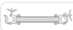
FRAME SECURING LOCK (FOR CRANE LIFT)
